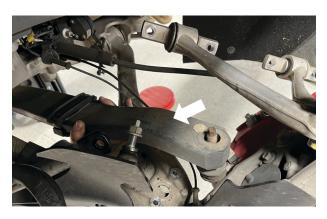
Fig. 12: Remove the leaf spring.
