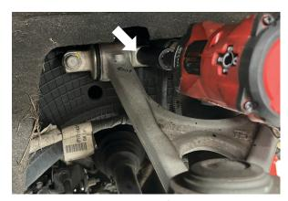
Fig. 23: Remove upper control arm.
