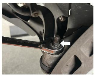
Fig. 4: Remove the outer tie rod from the steering arm.
