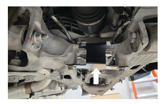
Fig. 28: Install reservoir mounts.
