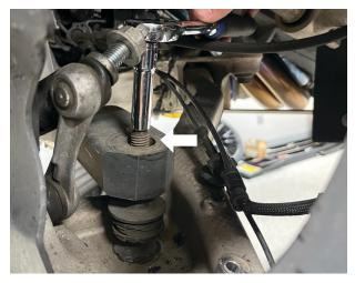
Fig. 10: Loosen the jack screw until the pad is touching the leaf spring.
