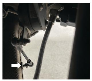
Fig. 36: Install the position sensor; hose routed behind sensor.
