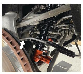
Fig. 30: Emergency brake line clearance.
