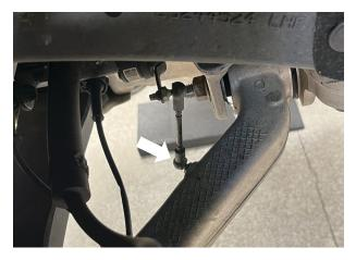
Fig. 1: MagnaRide: detach the factory position sensor.
