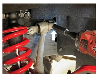
Fig. 15: Torque the upper control arm bolts to OEM specifications.
