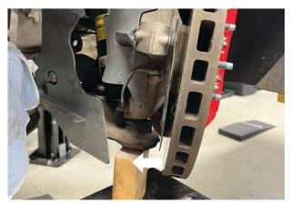
Fig. 5: Support the suspension.
