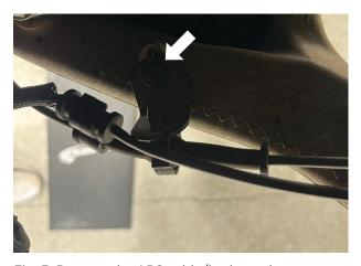
Fig. 3: Remove the ABS cable/brake pad wear sensor bracket.
