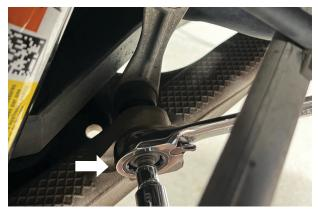
Fig. 22: Disconnect sway bar link.
