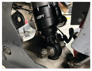
Fig. 14: Install the OEM shock mount bolts into the lower control arm.
