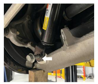
Fig. 24: Remove stock lower shock bolt.
