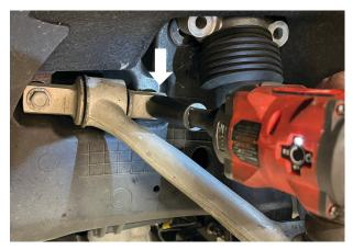
Fig. 8: Remove the upper control arm bolts.
