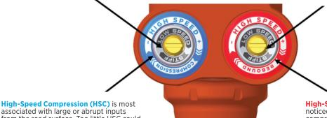
High-speed Compression (HSC) is most associated with large or abrupt inputs from the road surface. Too little HSC could cause the dampers to bottom over bumps and square edge inputs. Too much HSC can lead to harshness or being pushed off line by large inputs such as track curbing. Adjust with a 17 mm socket/wrench.
