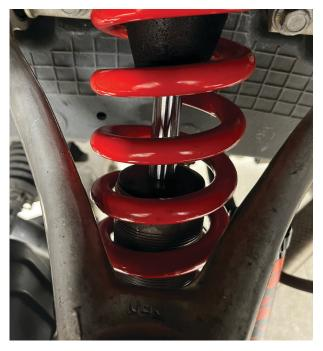
Fig. 17: Center the spring between the upper control arm legs.
