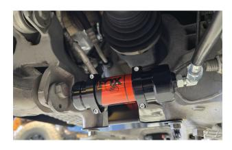
Fig. 35a: Reservoir and hose clearance.
