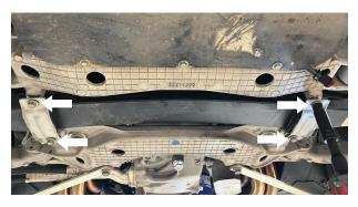
Fig. 11: Alternately and incrementally loosen the leaf spring mounting bolts.
