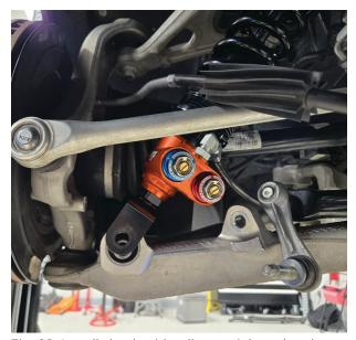
Fig. 29: Install shock with adjusters inboard and toward rear of vehicle.
