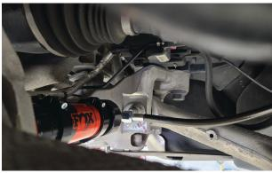
Fig. 35b: Reservoir and hose clearance.
