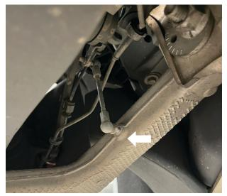
Fig. 21: Remove the position sensor.
