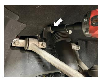
Fig. 7: Remove the upper shock bolts.
