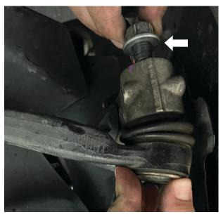
Fig. 16: Reinstall the tie rod end.
