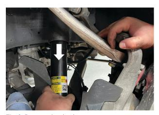
Fig. 9: Remove the shock.
