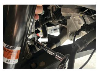
Fig. 2: Remove the sway bar.
