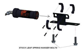
Fig. 33: Exploded view of reservoir/bracket/clamp assembly.
