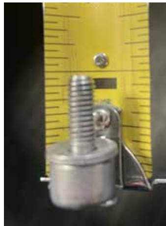
Figure B: Modified bolt after removing 1/16" from the tip
