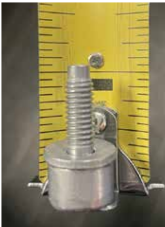
Figure A: Torx head Bolt with a longer unthreaded tip
