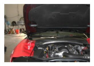
**Step 2:** Remove the OEM factory hood by removing the bolts/nuts attaching it to the hinge. (Note: You may have to remove any garnishes that are part of the OEM hood). You will need help from a partner to hold the hood while you are unbolting it.
