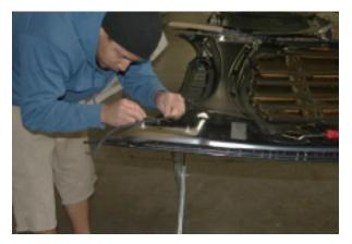
**Step 11:** Transfer the windshield hose and its frame over to the carbon hood. It may be necessary to enlarge the mounting points - you can do this by using a small file.
