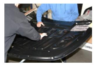
**Step 9:** Place the OEM heat shield on the carbon hood and proceed to reinstall the heat shield clips taken off in Step 4. \*It may be necessary to enlarge the holes on the hood's skeleton. These are purposefully smaller than OEM to ensure a snug fit.\*
