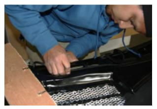
**Step 12:** In some cases, depending on the vehicle you have, you may have to/want to transfer your OEM striker onto your new carbon fiber hood. To do this, simply unbolt the striker and screw it onto the carbon hood.
