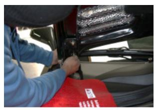
**Step 13:** Before closing the hood, make sure the fenders are clear and that there are no tools left in the engine bay. Carefully close the hood. Slamming the hood may cause it to crack. Check alignment of the hood and latch. If satisfactory, the hood installation is complete.
