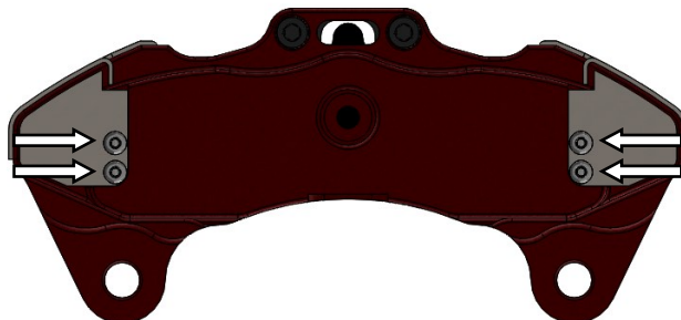
Figure 5. Bleeder guard installation
