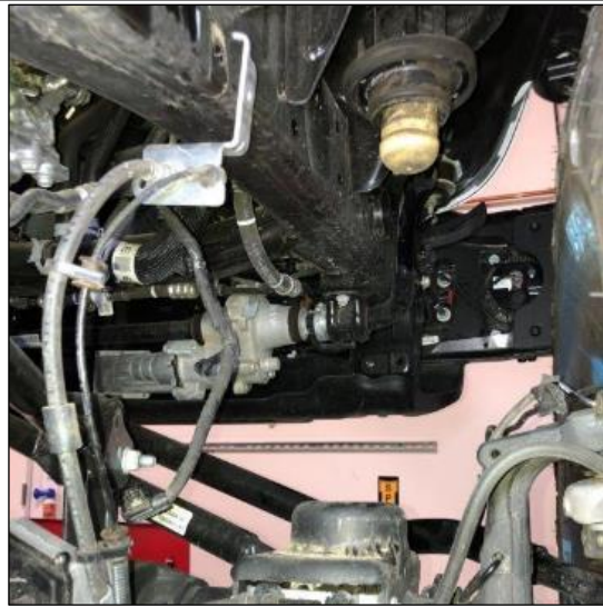
Figure 11: Passenger Side spring removed
