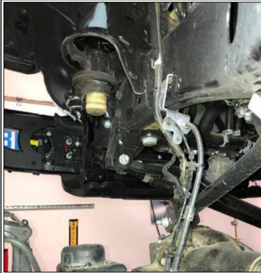
Figure 10: Driver Side spring removed
