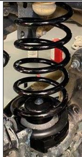
Figure 13: Driver Side bumpstop spacer and spring installed
