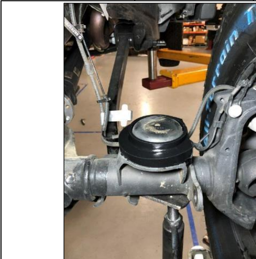
Figure 12: Driver Side lower isolator installed
