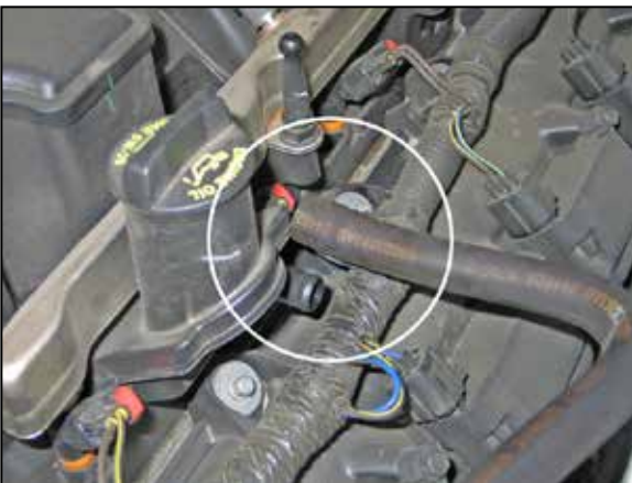
5. Disconnect the crankcase vent hose from the port on the valve cover.
