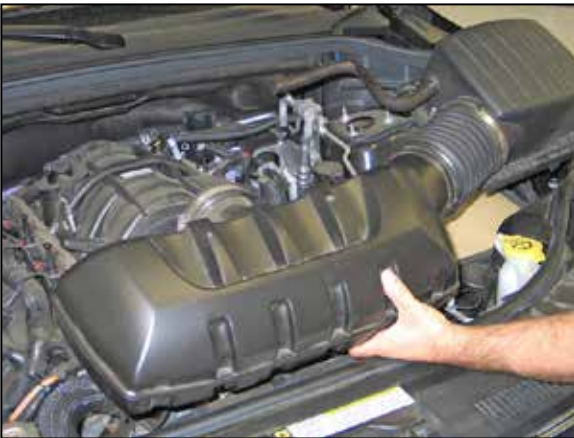
7. Remove the upper airbox and intake tube assembly.
