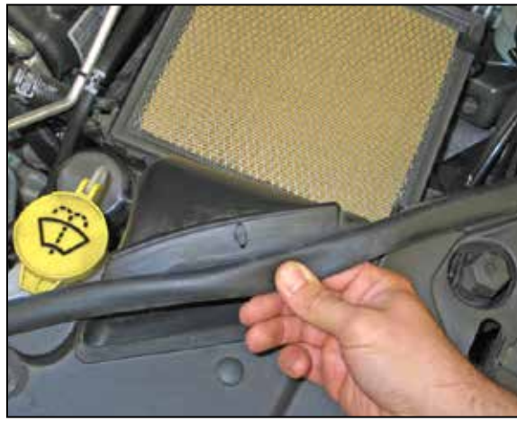
8. Unhook the sealing trim from the fresh air intake scoop and keep clip.
