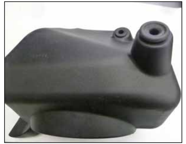
12. Install the 3 grommets from step 10 into the new K&N airbox.
