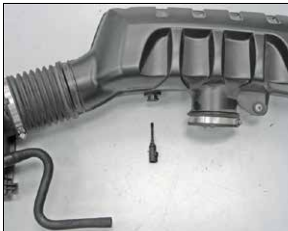
11. Release the locking tab and then remove the inlet air temperature sensor from the factory intake tube by twisting counter clockwise.
