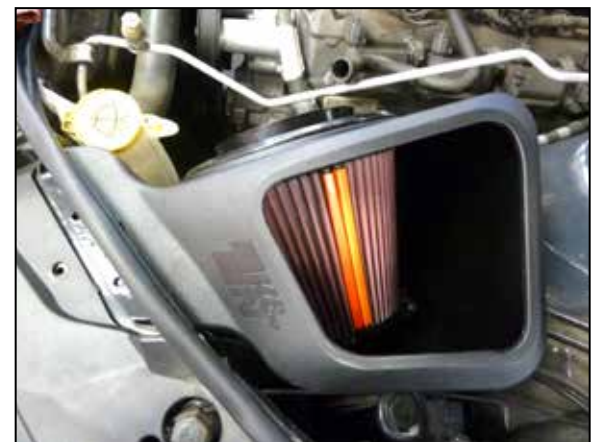
15. Install the airbox assembly into the vehicle and position to the original airbox mounting studs.
