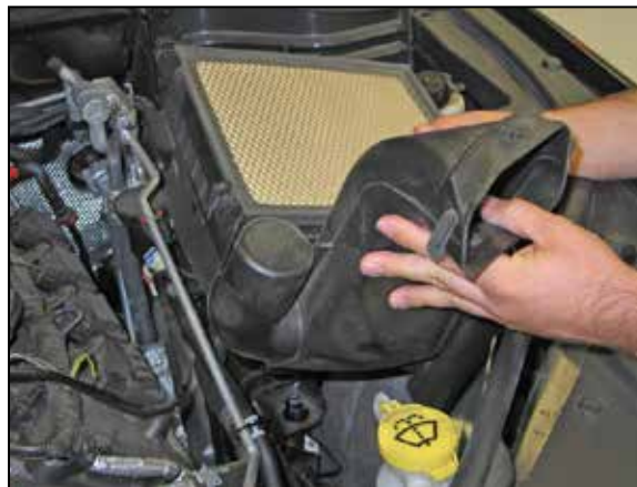
9. Lift up the lower airbox to dislodge it from the mounting grommets and then remove the lower airbox from the vehicle. Some vehicles may have a power steering line attached to the air box than will need to be unhooked.
