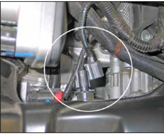
4. Disconnect the inlet air temperature air sensor electrical connection.
