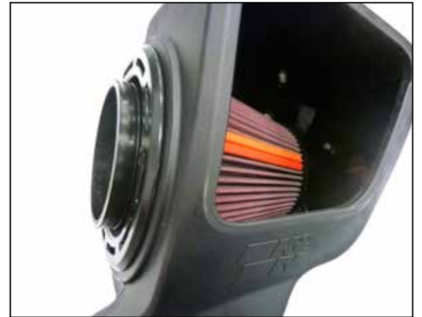
14. Install the air filter into the K&N airbox.
