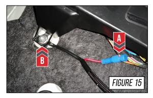
Located next to the box location is a grommet that is directly over the valve motor on the SwitchPath™ Exhaust system.
