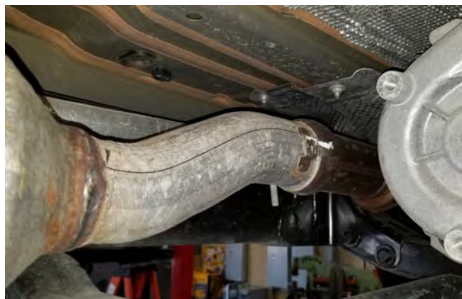
Detail 7: OEM catback connection
