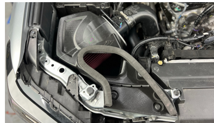
Figure 3: 3D printed Mishimoto intake prototype
