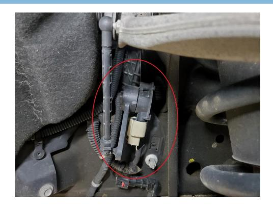
2. Disconnect Ride Height Connector from Sensor by unlocking red lock tab by pulling down or pushing down with flat head screwdriver. Then squeeze release tab and disconnect connector.
