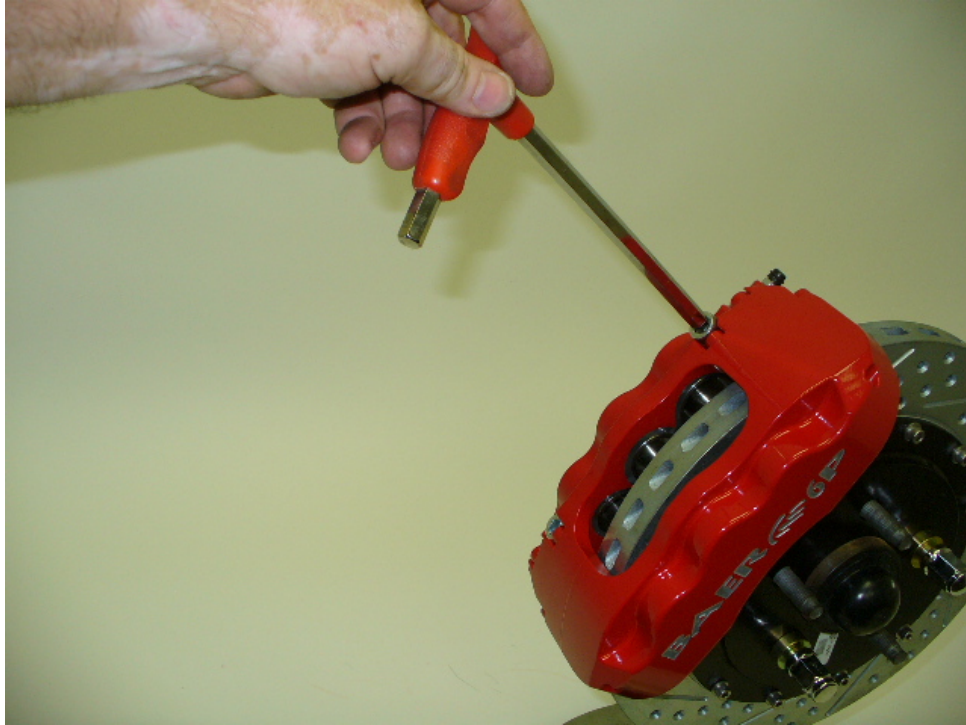
Pro Plus caliper installed without pads.
