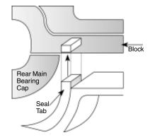
REINSTALL OIL PANTO ENGINE. Fel-Pro recommends the replacement of pan bolts and lock washers for all applications. Application with pan bolts shorter than 5/8" require the use of longer bolts. Torque bolts to the following specifications: 8 ft.lbs (10.7 Nm.) = 1.4" x 20 bolts (rail) 18 ft.lbs (24.3 Nm.) = 5/16 x 18 bolts (corners). Over-torquing can distort the oil pan and cause leakage.
