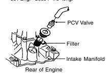
**IMPORTANT:** 1986 and later Ford 5.0L applications, require the replacement of the crankcase breather filter, located under the PCV Valve. If the filter is not replaced the filter can get clogged with carbon and sludge resulting in increased crankcase pressure, intake manifold end seal leakage, timing cover or rear main seal leakage.
