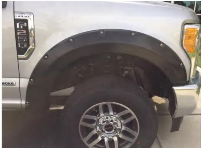
**STEP 6:** Place the Fender Flare onto the vehicle and fit into the correct position following the contours of the body. Ensure the slots in the part align with the holes in the fender from the previously removed 7/32" socket head screws.
