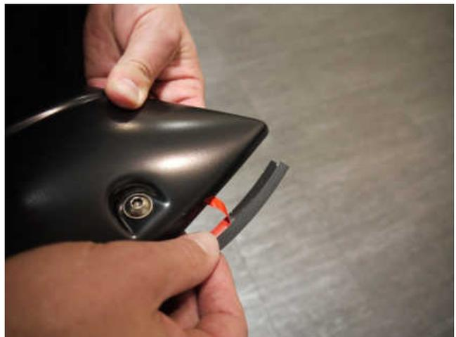
**STEP 2:** Attach the included rubber seal to the Fender Flares. Peel back 2" of the adhesive backing and position on the Fender Flare. Attach the double sided tape to the inside of the Fender Flare, peeling back a few inches at a time. Ensure pressure is used to secure rubber seal to Fender Flare edge. Attach rubber seal along all areas the Fender Flare will make contact with the vehicle body.
