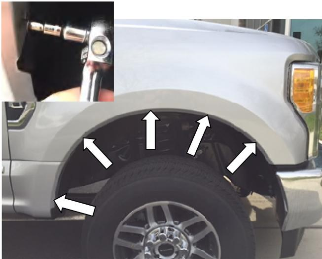
**STEP 5:** Remove all five (5) 7/32" socket head screws and retain for installation of Fender Flares.
