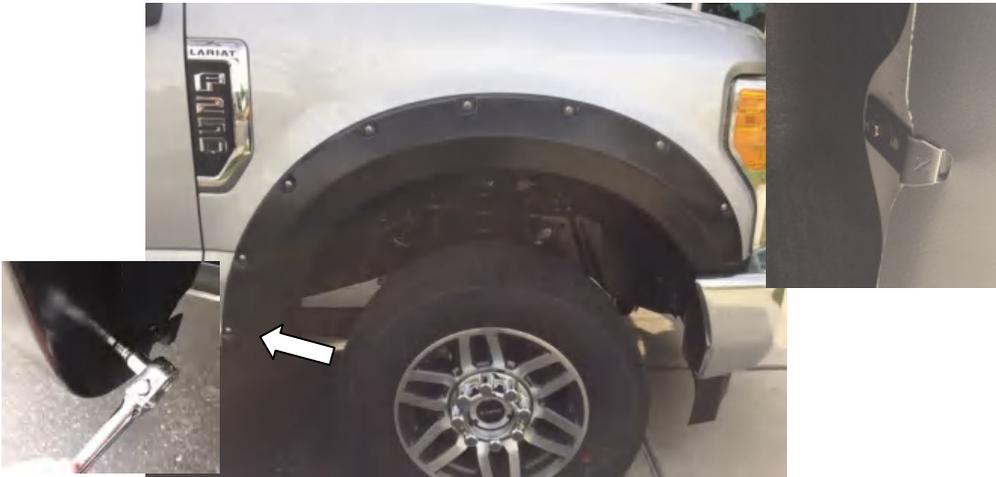
**STEP 7:** Loosely reinstall the lowest rear 7/32" socket head screws through slot in the Fender Flare to the vehicle. Make sure the screws are securely engaged to the vehicle fender. Install provided Long Attachment Clips in remaining four (4) Fender Flare Slots. Loosely reinstall remaining 7/32 in socket head screws. Ensure part is still in the position of best fit and extrusion is in correct position before hand tightening all screws.
