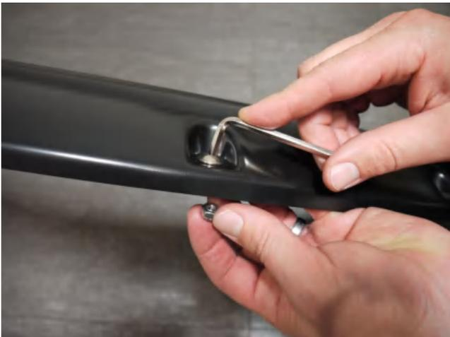
**STEP 8:** Attach the bolts and nuts to each Fender Flare using a 3/16" Allen key and a 10mm wrench/socket (wrench /socket and Allen key not supplied). Ensure inside of Fender Flares where the rubber seal is attached is clean, using the alcohol wipes provided. Wipe away any residue with a dry clean cloth.
