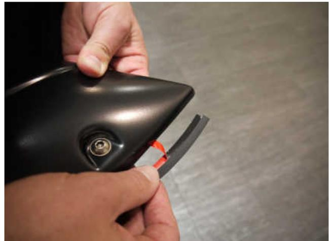
**STEP 9:** Attach the included rubber seal to the Fender Flares. Peel back 2" of the adhesive backing and position on the Fender Flare. Attach the double sided tape to the inside of the Fender Flare, peeling back a few inches at a time. Ensure pressure is used to secure rubber seal to Fender Flare edge. Attach rubber seal along all areas the Fender Flare will make contact with the vehicle body.
