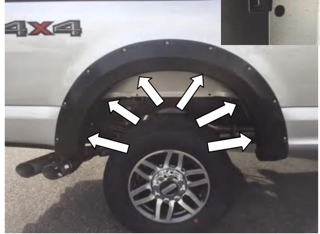
**STEP 10:** Clean the body areas where the Fender Flares will make contact. A light misting on fender using a soap and water solution can aid in proper rubber placement.
