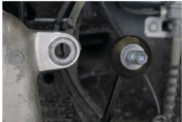
Fig. 3: Disconnect the sway bar end link.
