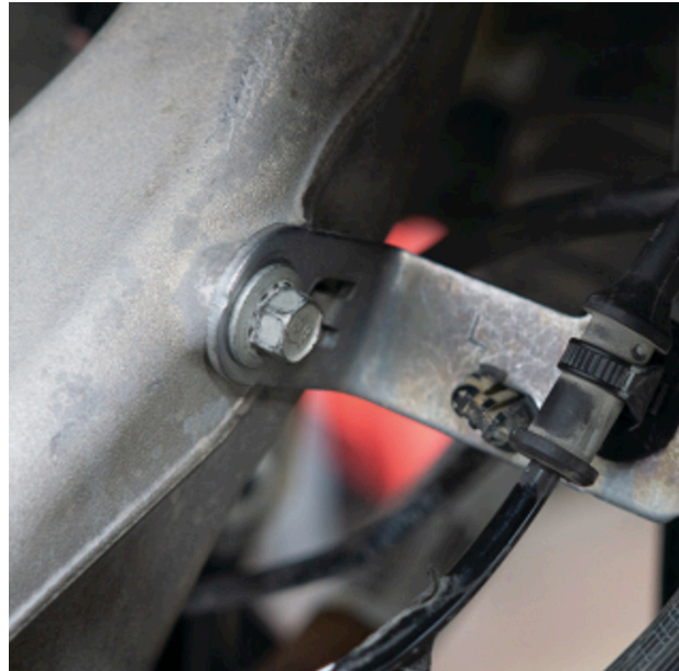
Fig. 12: Install brake hose bracket.
