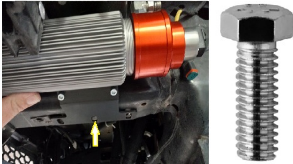
Fig. 15: Bolt installed to hold reservoir assembly for alignment and 2nd bolt hole drilling.
