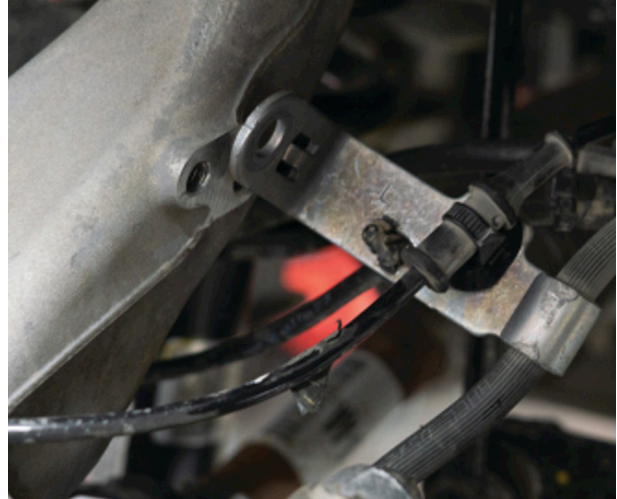
Fig. 1: Disconnect brake line bracket.
