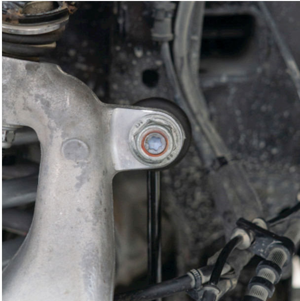
Fig. 11: Install sway bar end link.
