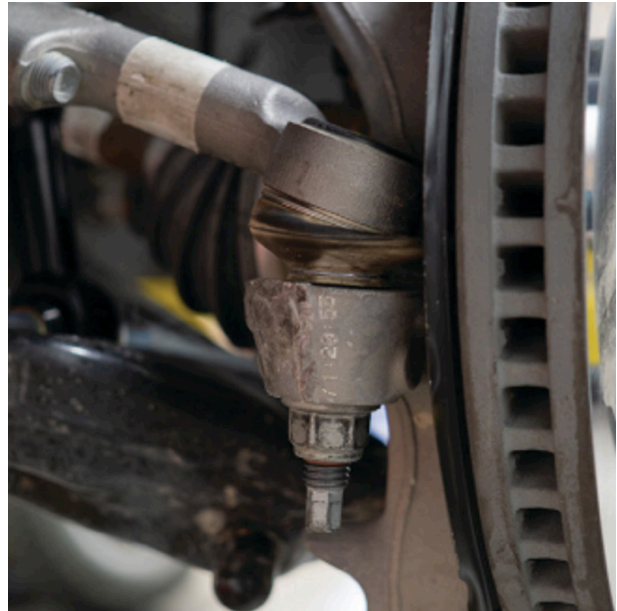
Fig. 10: Install tie rod end link.
