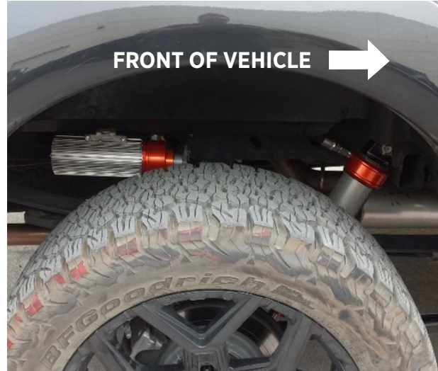
Fig. 21: Right rear shock orientation.
