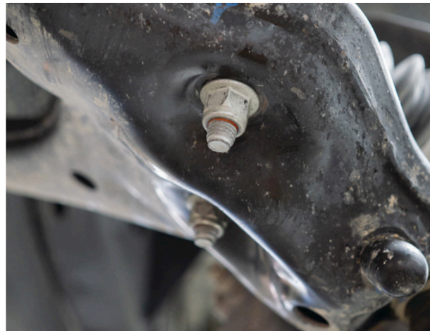
Fig. 7: Remove the bar-pin nuts.
