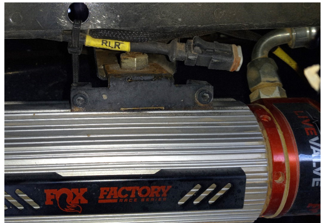
Fig. 25: Reservoir assembly attached to bed frame channel.
