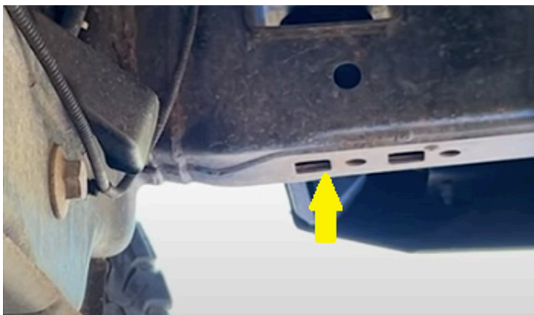
Fig. 14: Insert clip nut into rear most frame mount provision.
