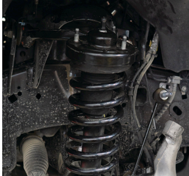
Fig. 6: Release the coil-over.
