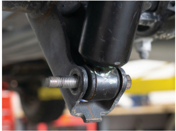
Fig. 20: Remove lower shock mount bolt.
