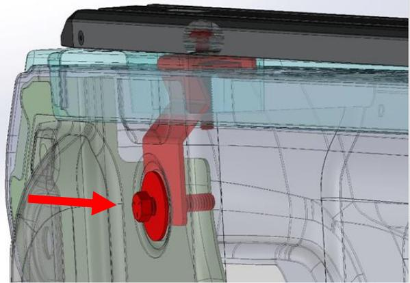
18. Align the front end cap on the Tec Skin extrusion so that it is flush with the bed cap end, as shown. Position the extrusion in the desired final position.
