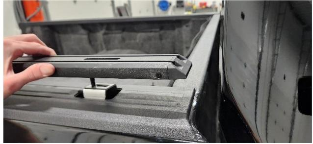
14. Adjust the position of the threaded plate to set the stake pocket bracket to an appropriate height so that the nut clip on the bracket aligns with the hole in the sidewall of the bed.
