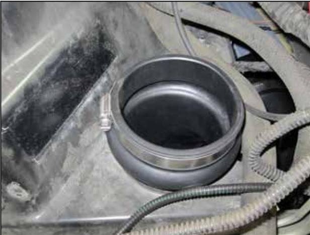
b. Loosely install a #56 hose clamp over the upper opening of the elbow hump hose.
