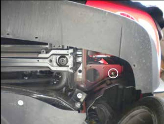
b. From underneath the car, install the M8 rubber mount through the slotted hole in the sheet metal, secure with 1 M8 washer and nut. Do not completely tighten the M8 nut, this will allow room for adjustment.
