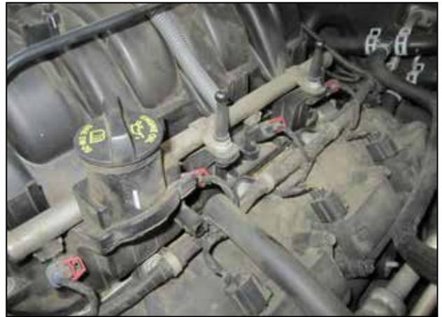
b. Pull to remove the crank case breather hose from the nipple on the head cover.
