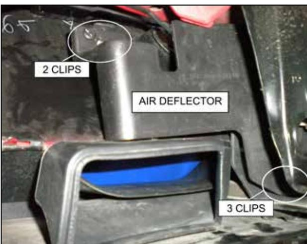
i. For maximum performance from your intake system, you may choose to remove the air deflector. If equipped, the air deflector will be located behind the lower grill on the driver side. Removing this will provide additional cold air flow to the air filter.
