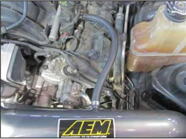
f. **For Most Applications:** Install the supplied 1/2" ID hose between the crank case vent on the head cover and the nipple on the upper intake pipe. Secure the 1/2" hose with two small hose clamps.
