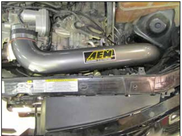
e. The lower end of the pipe should be inserted into the rubber coupler to a depth of about  $\frac{3}{4}$ " to 1". Slide the pipe all the way into the throttle body coupler until it bottoms out. Once proper fitment is achieved, tighten the two remaining hose clamps.
