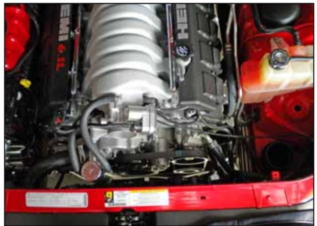
d. Pull the rubber inlet hose off of the throttle body, then lift and remove the OEM air box assembly.
