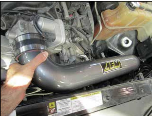
d. Insert the lower end of the upper intake pipe into the rubber coupler, and then carefully angle the other end into the throttle body coupler. The hose clamp on the rubber coupler may need to be extra loose to achieve this.
