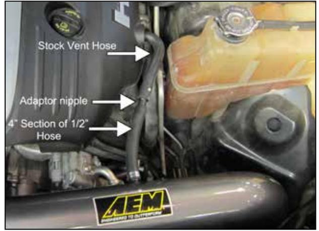
g. **On some 5.7L engines:** Connect the stock crank case vent hose to the supplied plastic adaptor nipple. Connect a 4" section of the 1/2" ID hose onto the other end of plastic adaptor nipple. Connect the hose to the intake pipe and secure with the small hose clamps as shown.
