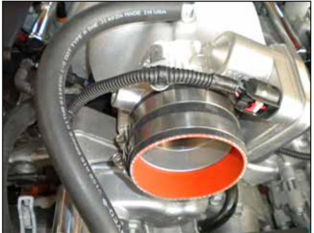
c. Install the silicone coupler and two #56 clamps onto the throttle body. Slide the coupler all the way onto the throttle body and secure it by tightening one of the #56 clamps.
