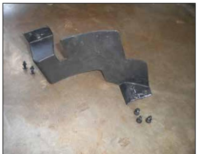
j. To remove the air deflector, remove the five plastic rivets securing it to the fascia. The rivets can be removed by pulling the center pin out from the back side of the rivet.
