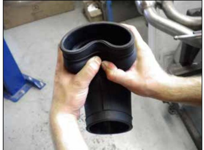
c. Hold the rubber coupler as shown, squeeze the hump end of the coupler to collapse it into itself.
