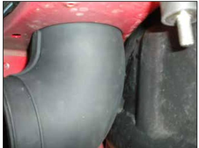
e. Make sure that the hump is all the way through the hole, then release the coupler and manipulate it until the sheet metal "snaps" into the groove in the coupler.
