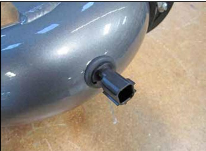
h. Carefully install the IAT sensor into the grommet.
