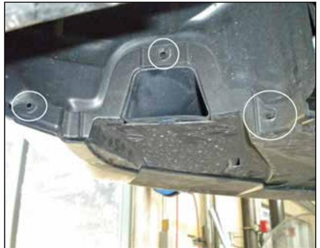
f. In the wheel well area on each side, remove the 3 clips securing the belly pan.
