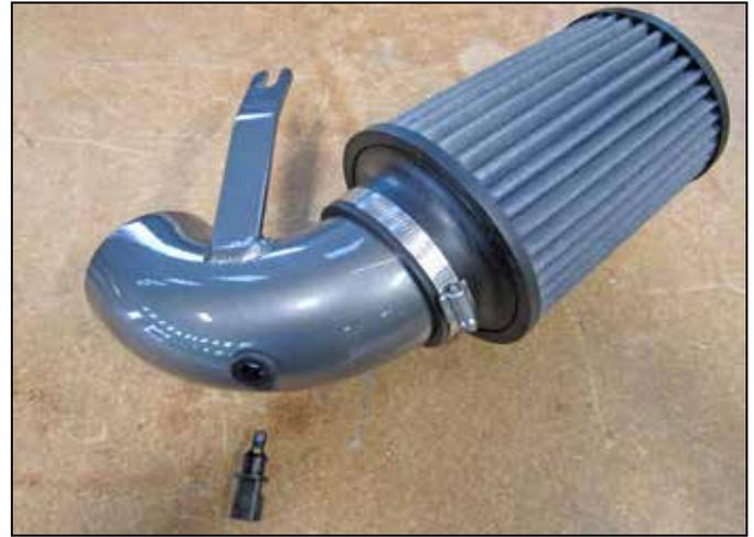
g. Install the grommet into the lower pipe and attach the filter with one #56 clamp as shown.
