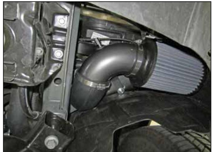
i. Install the lower pipe assembly as shown using one M8 washer, one M8 nut, and one #56 clamp.
