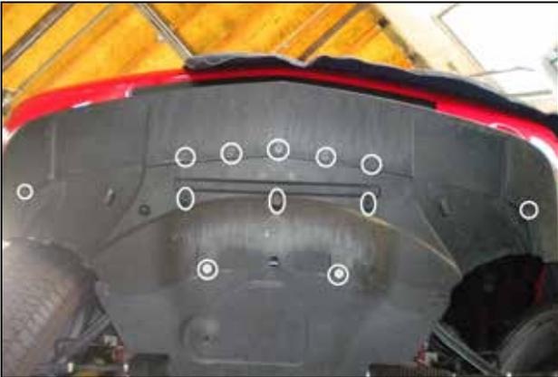
h. Install the belly pan with the 9 clips, 7 screws, and 2 bolts removed in steps 2f and 2g.
