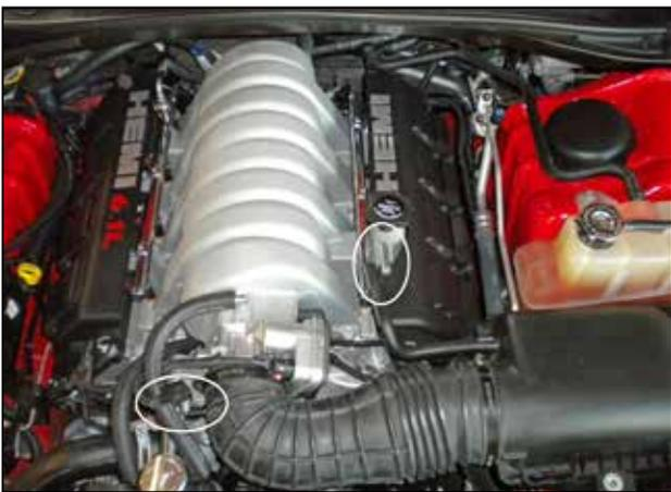
c. Unplug the IAT sensor. To unplug the IAT sensor, slide the red tab back to unlock the latch on the plug, then press in on the latch and pull the plug off of the sensor. For "grey" tabbed connectors, push the top of the gray tab in and simply pull the connector off.
