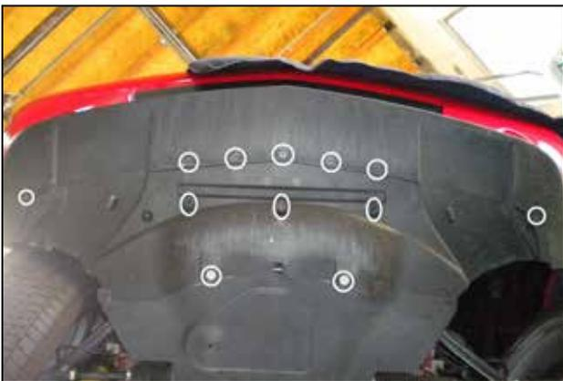
g. From underneath the car, remove: 3 clips, 7 screws, and 2 bolts from the belly pan. (May vary with each vehicle.)
