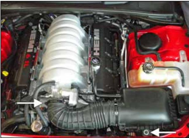
a. Remove the bolt securing the OEM air box and loosen the hose clamp at the throttle body.
