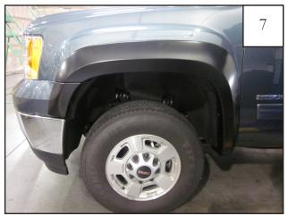
**OPTIONAL BUMPER PIECE:** Completed front flare installation.
