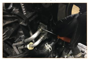
11. Remove the bolts securing the top of the radiator to the radiator support (2x 10mm bolts).
