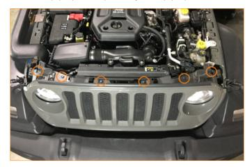
02. Pull outward on bottom of grille to remove it from the vehicle.
