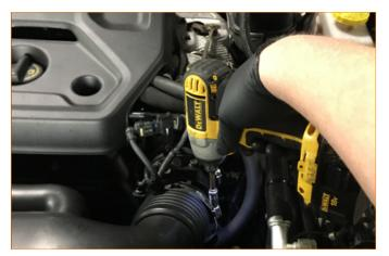
05. Unbolt the intake tube from the fan shroud (2x 10mm bolts).
