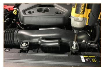
**06.** Remove the vacuum lines from the intake air box and then remove the air intake assembly from the vehicle. (2x vacuum lines)
