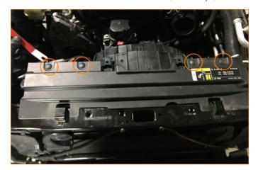
**08.** Disconnect the radiator fan harness (1x electrical connector and 1x tree clip).
