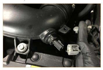
04. Loosen the air intake tube connection (1x worm gear clamp).
